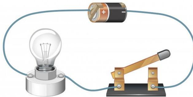
**A series circuit created from a battery, a switch, and a light bulb**
